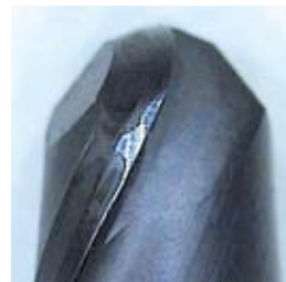
Competitor's diamond tool: after 4850m cutting length
