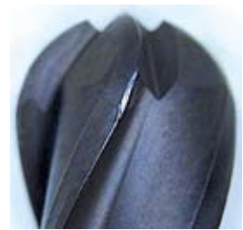
IDI diamond tool: after 10500m cutting length
