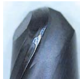
Competitor's diamond tool: after 4850m cutting length
