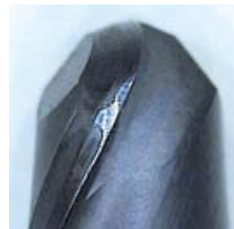
Competitor's diamond tool: after 4850m cutting length
